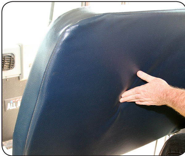
The edge of the rigid foam inside the cover of a Barrier or a 2/3 Seat extends beyond the vertical support leg, which is offset from the aisle-side of the seat.
