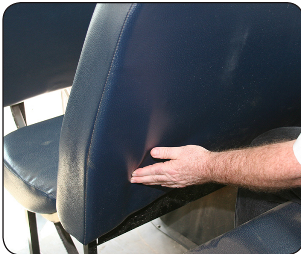
The pad of a regular seat back also has rigid foam pieces, but they do not extend as far from the aisle-side of the seat, because the vertical support leg is not offset.
