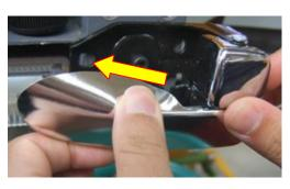
6. Turn back the upper edge of the protection wrap toward the back of the door inside handle, then stretch it tight.
