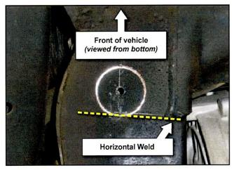
Referencing the dashed line, measure thirty (30) mm from the outer horizontal weld (dashed line) and mark this location. From this new reference mark, measure ten (10) mm forward from this position and mark this location as the center point of the drilling. Drill this location using the forty (40) mm hole-saw (Drill speed recommendation: 380 ~ 470 rpm).
