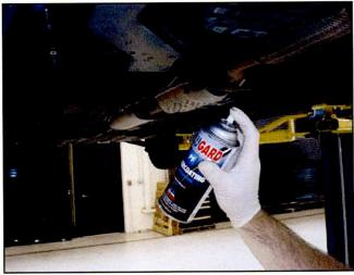
13. Cover all four (4) of the 40mm access holes with the hole plugs listed in the parts information section and apply a small amount of undercoating across the plugs.
