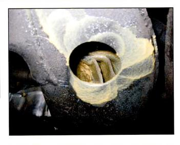
12. Spray undercoating on the underside of the subframe near the four (4) 40 mm access holes and 8 mm drain holes. Do not spray the entire subframe with undercoating.
