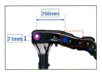
8. Place the LH and RH templates against the underside of the subframe, just parallel to the control arm with the arrows pointing forward. Align the outlines on the templates to the outboard shape of the subframe. Ensure proper orientation of the front (Frt) alignment of the templates for left/right. Use a grease pen to mark through the two holes on each template.
