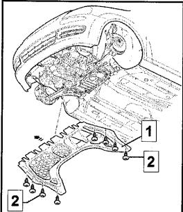
Reinstall noise insulation cover -1- and screws
