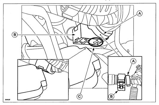
3. Refasten the lower harness anchor if unfastened in PROCEDURE "D" - INCREASING WORK SPACE.
