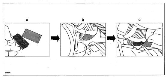
3. Using 35 inches of electrical tape, wrap the harness to completely cover the butyl taped area as shown.
