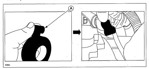
4. Perform PROCEDURE "B" - INSTALL EMISSION HARNESS PROTECTOR CLIPS.
