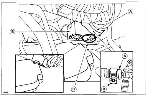
3. Refasten the lower harness anchor if unfastened in PROCEDURE "D" - INCREASING WORK SPACE.
