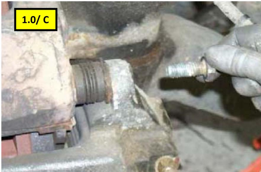
12. Move caliper assembly away from rotor.
