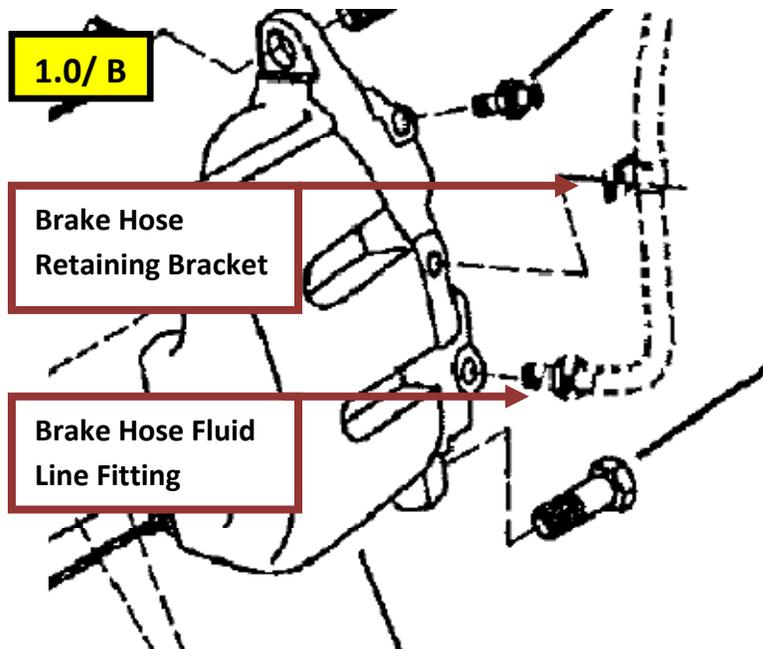
9. Disconnect brake hose fluid line fitting from caliper and cap off to prevent brake fluid leakage or contamination in the line. Do not allow the brake line hose to become pinched or kinked during the remedy procedure. (View Illustration 1.0/ B)
