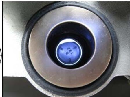
The pistons have the letter "B" molded in three locations at the bottom of the piston.
