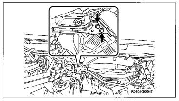
b) Install the bracket with the 2 bolts.
