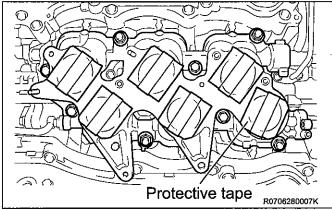
Place protective tape over the intake manifold openings to prevent foreign objects from entering.
