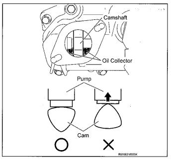
i) Turn the crankshaft until the flat of the cam is facing the cylinder head cover's fuel pump attachment hole, as shown in the illustration.
