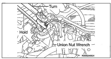
Using a 19 mm union nut wrench, connect the fuel pipe.
