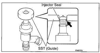
k) Slowly slide SST (guide) towards the tip of the injector. When the injector contact surface of SST (guide) aligns with the seal (injector tip side) as shown in the illustration, hold the position for 5 seconds or more to fully align the seal into the injector groove.
