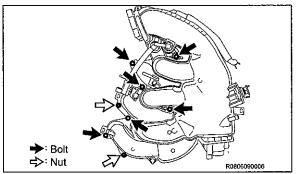
I) Using a hexagon 5 mm, remove the 6 bolts, then using a 10mm socket remove the 2 nuts.
