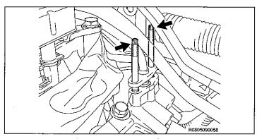
d) Hand tighten the 2 stud bolts to the delivery pipe bolt attachment holes. (torx® side up)
