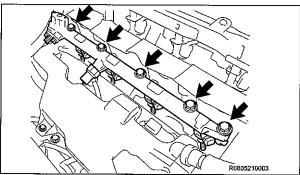
c) Remove the 5 bolts and delivery pipe.
