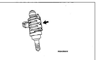
c) Remove the nozzle holder clamp from the injectors.
