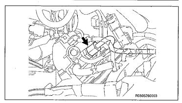
g) Loosely install the No. 3 fuel pipe sub-assembly to the fuel pump assembly.
