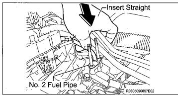
e) Press the fuel pipe and delivery pipe together by hand until there is no gap between them.
