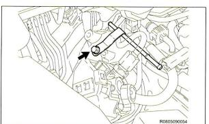
Remove the bolt, and disconnect the No.1 fuel pipe subassembly.
