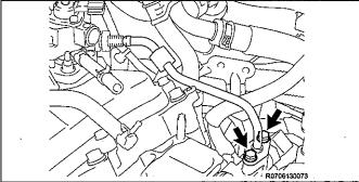
b) Remove the 2 bolts on the delivery pipe side.
