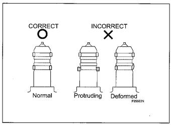
After installing the seals, check that the seal is not scratched, deformed or protruding from the injector groove.
