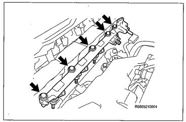
c) Install the No. 1 delivery pipe with the 5 bolts.
