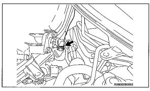
h) Disconnect the ventilation hose from the intake manifold.
