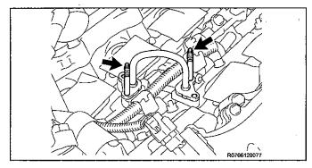
b) Hand tighten the 2 stud bolts to the delivery pipe. (torx® side up)
