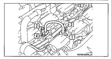
Clean the screw holes of dirt and gasoline, and then insert and tighten the 4 bolts in the order shown in the illustration.
