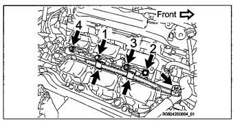
g) Install the fuel delivery pipe by uniformly tightening the 2 bolts and 2 nuts in several passes in the order shown in the illustration.
