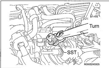
f) Use SST or equivalent, securely tighten the fuel pressure pulsation damper LH.
