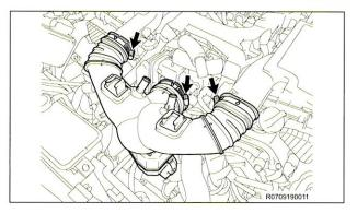
c) Loosen the 3 hose clamps, and remove the intake air connector pipe.
