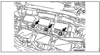
e) Remove the 3 injector vibration insulators from the cylinder head.
