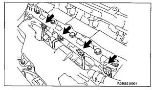
b) Disconnect the 4 electrical injector connectors.
