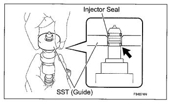
i) Slowly slide SST (guide) towards the tip of the injector. When the injector contact surface of SST (guide) aligns with the seal (injector connector side) as shown in the illustration, hold the position for 5 seconds or more to fully align the seal into the injector groove.
