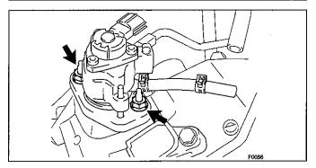
c) Remove the 2 nuts from the fuel pump.
