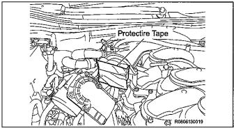
c) Place protective tape over the surge tank opening to prevent foreign objects from entering from the old gasket above.
