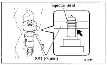
e) Using SST (holder), gently press downward on the injector seal (injector connector side). Then slowly slide SST (guide) towards the injector tip to settle the seal into the injector groove.
