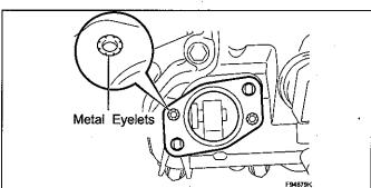
Install a NEW fuel pump insulator to the cylinder head cover.
