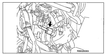
g) Loosely install the No. 2 fuel pipe sub-assembly to the fuel pump assembly.
