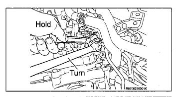
a) Fix the union bolt on the fuel pump side in place with a 21 mm wrench. Using a 19 mm union nut wrench, loosen the union and remove the fuel pipe.
