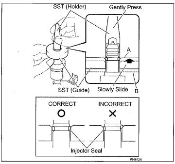
b) Apply engine oil to the injector contact surface of SST (guide). Then attach SST (guide) to the injector with the tapered inner portion facing the tip of the injector, as shown in the illustration.
