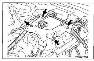
q) Remove the 4 nuts, and disconnect the engine wire.
