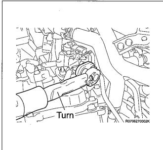
b) Using a 19 mm union nut wrench, connect the fuel pipe.
