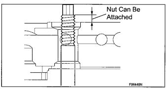
f) Install the fuel delivery pipe until the screw threads protrude enough so that a nut can be attached.
