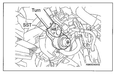
e) Use SST or equivalent, securely tighten the fuel pressure pulsation damper RH.
