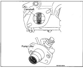
k) Apply a coat of engine oil to the pump activation cam and pump lifter part.
