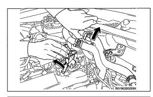
d) Remove the fuel pump and fuel pump insulator.
