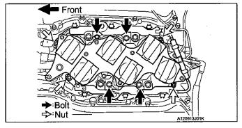
d) Remove the 4 bolts, 4 nuts, intake manifold and gasket.
