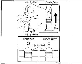
j) Using SST (holder), gently press downward on the injector seal (injector tip side). Then slowly slide SST (guide) towards the injector tip to settle the seal into the injector groove.
