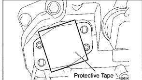
e) Place protective tape on the old insulator and place it over the head cover opening to prevent foreign objects from entering.
