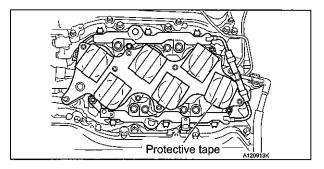
Place protective tape over the intake manifold openings to prevent foreign objects from entering.
