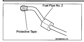
a) Place protective tape over the taper section of the No.2 fuel pipe's fuel pump to prevent damage.
