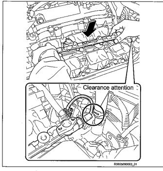
c) While gently raising the front of the delivery pipe, carefully insert the fuel delivery pipe on to the cylinder head's stud bolts. Do not allow the fuel pressure sensor and heater hose come in contact.
