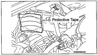
c) Place protective tape over the surge tank opening to prevent foreign objects from entering from the old gasket above.
