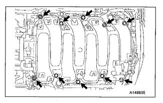
c) Using a 12 mm deep socket wrench, remove the 8 bolts and 2 nuts.
