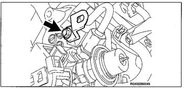
h) Install the bracket with the bolt.
