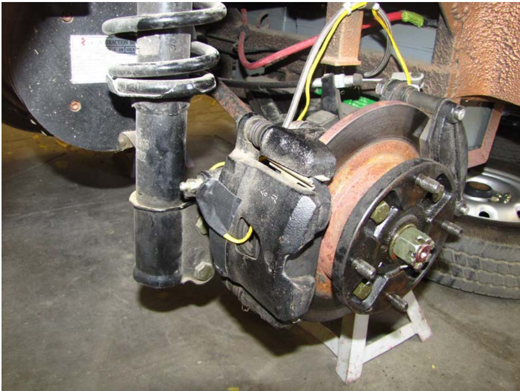
FIGURE 20. RIGHT REAR BRAKE WITH THERMOCOUPLE INSTALLED
