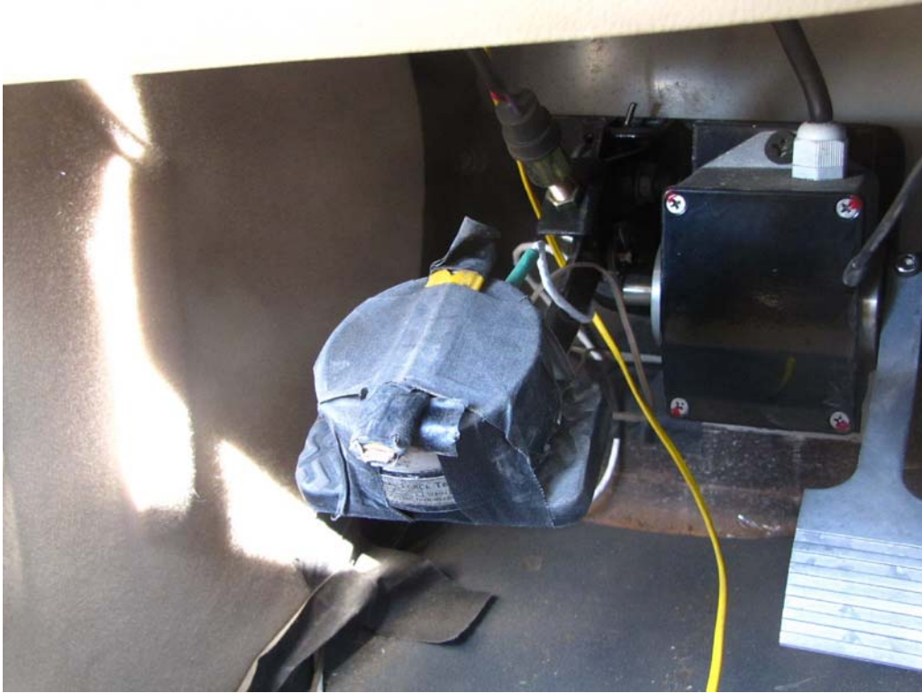
FIGURE 13. BRAKE PEDAL WITH LOAD CELL
