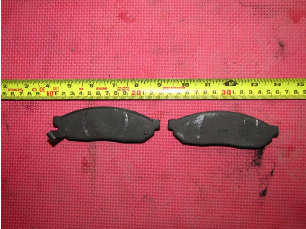
FIGURE 23. RIGHT REAR BRAKE PADS
