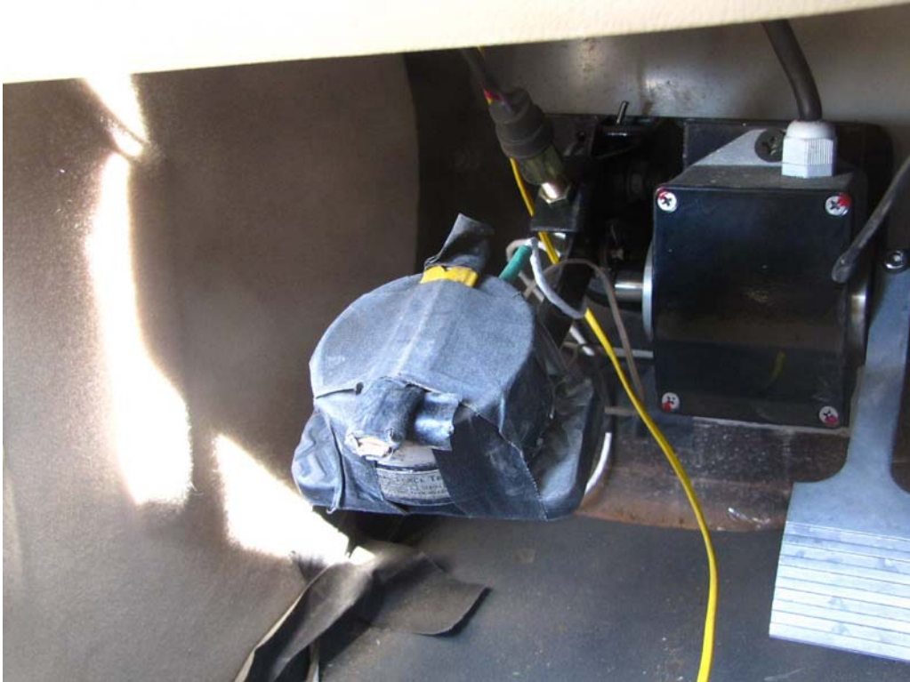
FIGURE 13. BRAKE PEDAL WITH LOAD CELL
