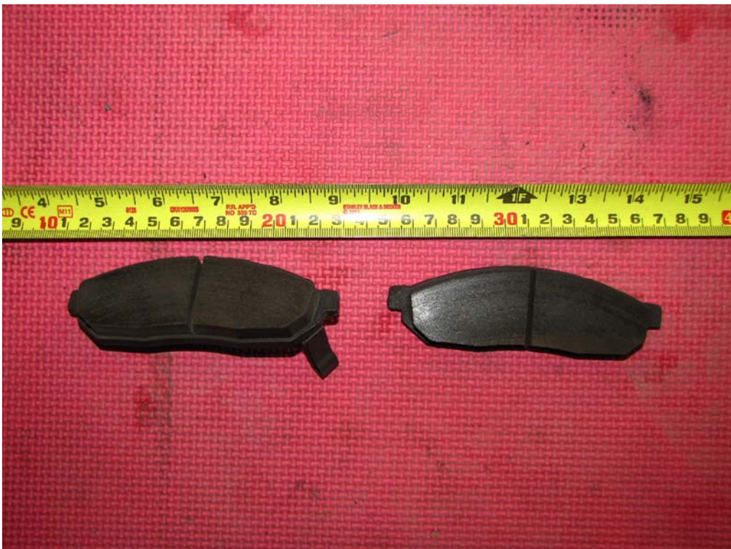
FIGURE 22. RIGHT REAR BRAKE PADS
