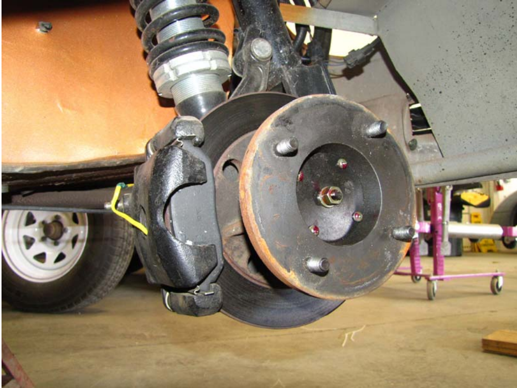
FIGURE 15. FRONT BRAKE WITH THERMOCOUPLE INSTALLED
