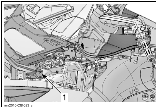
TYPICAL 1. Middle retaining screw
