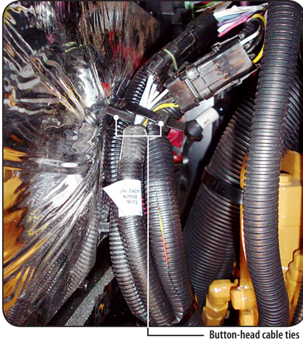
Area of possible cable damage against front edge of transmission cover plate
