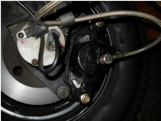
Fig. 5: Braided Stainless Steel Brake Line
