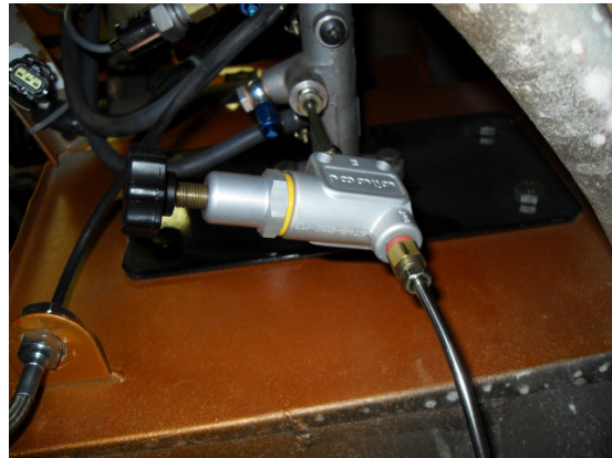
Fig. 6: Wilwood Proportioning Valve Part # 260-8419
