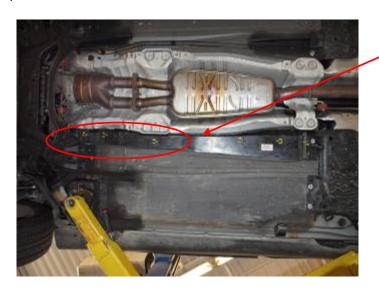
Inspect clips on front of fuel rail cover.
