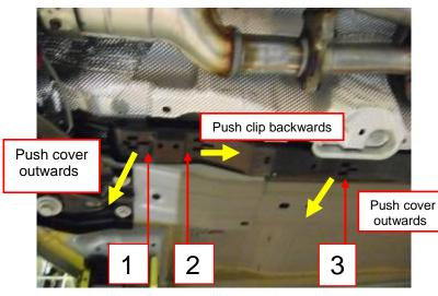
If clip 1 is not secure push the rail outwards to align over body stud.
