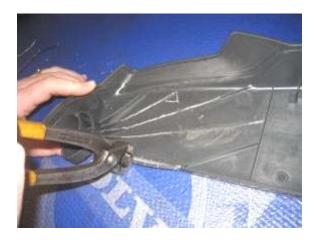
With the end cutting pliers cut off as much of the rib material from the back-side of the panel as possible.
