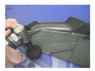
After cutting with the end cutters use a small grinding tool to remove the remaining rib material from the back-side of the panel as shown here.
