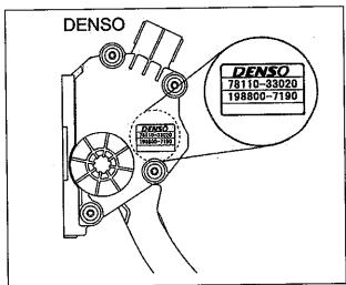
4. IDENTIFY AND REMOVE THE DENSO ACCELERATOR PEDAL ASSEMBLY
