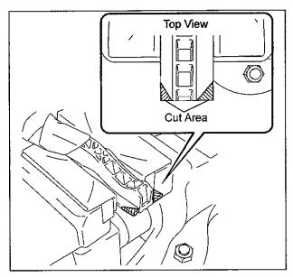
b) Using a reciprocating saw, cut the comers of the pedal.
