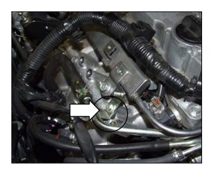
9. Torque the bolt securing Bracket A (small bracket) to 10 Nm ± 2 Nm (7.5 ± 1.5 ft/lb or 90 ± 18 in/lb).
