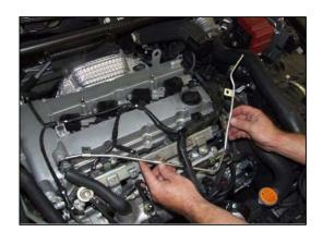
Loosen the hose clamps at both ends of the fuel return pipe and pull off the hoses. Then remove the three bolts securing the pipe and remove the pipe from the engine compartment.
