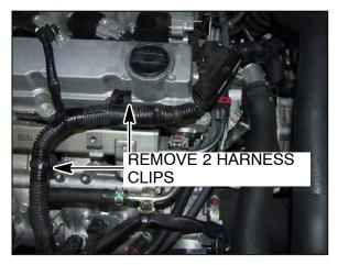
4. Remove the harness clips to access the fuel return pipe.
