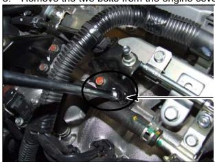
REMOVE ENGINE COVER BRACKET (2 BOLTS)
