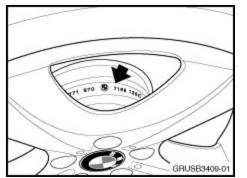
The stamping of the rear brake discs can be viewed by looking through the spokes of the alloy wheels. If there is any dirt or debris on the rear brake disc, clean the hub of the brake disc with a clean, dry, lintfree cloth.
