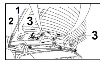
Reinstall three nuts -3- and torque to 6 Nm (4 lb-ft)
