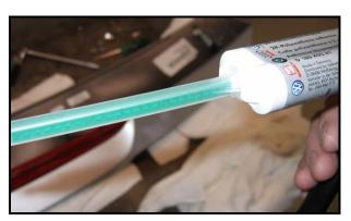
Remove the white and red protective caps from bonder and install mixing jet (D 001 001) onto bonder, as shown
