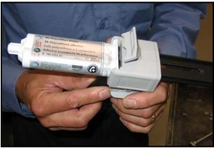
Fit bonder cartridge (D 180 KD2 A1) into VAS 5155, as shown
