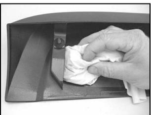
Clean and degrease all 3 areas of the attachments (for example, with cleaning solution D 009 401 04 – shop supply) and allow to completely dry
