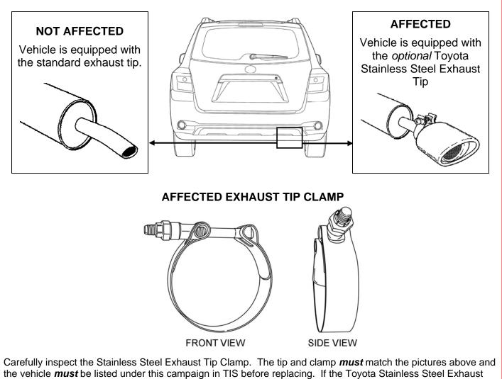
the vehicle **must** be listed under this campaign in TIS before replacing. If the Toyota Stainless Steel Exhaust Tip clamp appears to match the picture above but the vehicle is not listed as affected in TIS please call (310) 468-5516.
