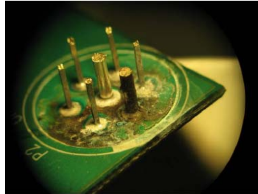
Corrosion advanced to a conductive condition
