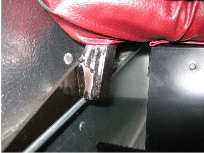
Figure 4: B1 Post test close up view of outboard attachment
