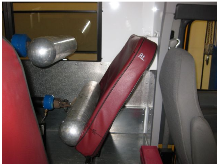
Figure 3: B1 Barrier Post-Test
