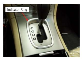
Remove the front console panel by gently pushing in on each tab (4) using a plastic trim tool.
