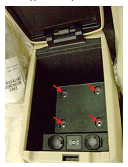
Gently pull the center console assembly rearward to disengage from the lower instrument panel. Carefully position center console assembly upward to gain access to G sensor.
