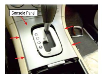
Remove the 2 screws that secure the front of the console.
