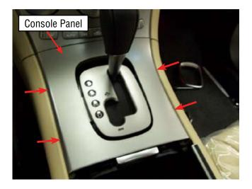
Remove the 2 screws that secure the front of the console.
