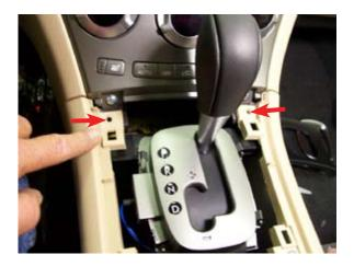
Remove the 4 bolts that secure the upper console pocket.
