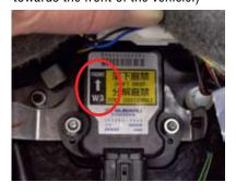
Incorrect Position (arrow is pointing towards the rear of the vehicle.)
