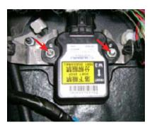
Reposition the G Sensor with the arrow pointing towards the front of the vehicle, install nuts and torque to 7.5 N-m (0.76 kgf-m, 5.53 ft-lb).
