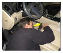
Push in, slightly pull down, and move the carpet slightly forward to gain a view of the G Sensor. Use a flashlight to verify the direction of the arrow on the G Sensor.
