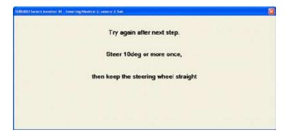
In either case, the display will go back to the function check sequence after a few seconds. Center the steering wheel and repeat the procedure.
