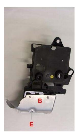
Install the heat guard B on the battery support using the three screws E
