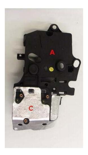
Install the adhesive protection C on the battery support A as shown in the picture.
