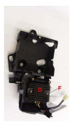
Install the voltage regulator D on the battery support using the two screws  $\mathsf{F}.$
