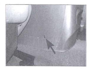
Lift up and remove the floor console assembly.
