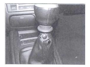
Remove the floor console forward and center mounting screws on both sides.
