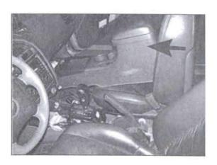
Using a clean dry cloth, wipe the airbag control module top surface near the connector to remove any dirt or contaminants.
