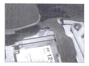
9. Make sure the vinyl cover is centered and extends over the edge of the airbag control module to shield the airbag control module wiring connector.
