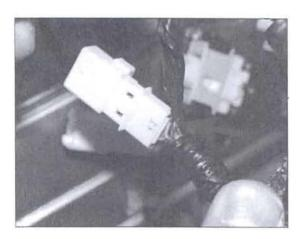
11. Using new electrical tape, tape the airbag floor wire, covering the connector and the end of the corrugated tube as shown in the photo.
