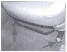
4. Slide the driver's seat fully forward and remove the 2 rear seat track mounting bolts.
