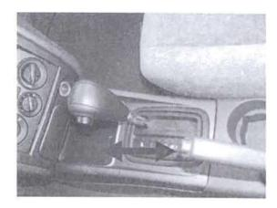
For manual transaxles, apply the parking brake and rotate the shift lever knob counterclockwise to remove. Lift and remove the console upper cover.
