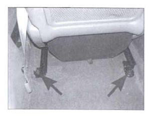
Tilt the driver's seat assembly rearward and disconnect the Buckle Switch, the Buckle Sensor and the side airbag (SAB) wiring connectors on the seat under frame.
