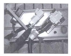
Remove the wrapped electrical tape over the airbag floor wiring connector and the corrugated tube.
