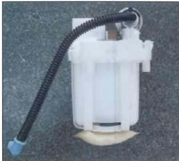
Fuel Pump Sub-assembly, Part No.: 31110 1D505QQK
