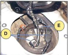
NOTE: Once fully reconnected, be sure to slide the collars of the quick connectors to the lock position.
