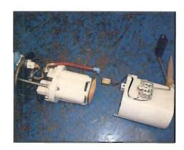
Remove the E-ring (N), and then remove the fuel pump plate (N1) from the fuel pump subassembly.
