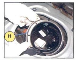
Remove the fuel pump assembly from the fuel tank.
