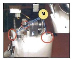
Separate the lower reservoir from the fuel pump assembly
