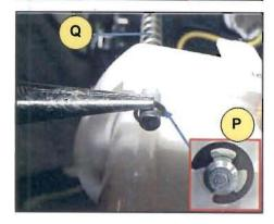
Reattach the lower reservoir to the installed new subassembly.
