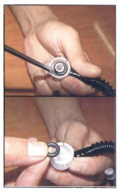
Install the output hose coupling and the fuel pump plate to the new fuel pump subassembly.
