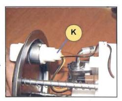
Disconnect the fuel pump wiring connector (L) from the fuel pump upper body.
