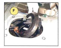
Using SST (G), unscrew the fuel pump plate cover (H) and remove the fuel pump plate cover.
