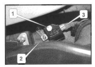
Attach locking cable -2- and secure clamping piece -3 - by tightening bolt -1-
