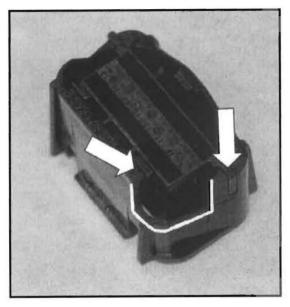
Tip: Take care not to cut off the guide and the retaining tab for the diagnostic connector (arrows).
