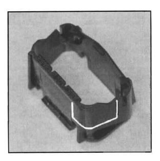
Carefully cut a section out of plastic mounting for diagnostic connector, as shown in illustration
