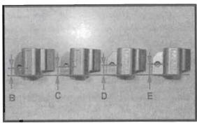
Tip: One of four adjusting pieces (part number 4D0713299 B, C, D, or E) with different hole alignments will now be used instead of elongated hole.
