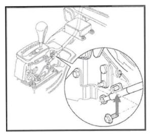
Tip: Elongated hole –arrow- will no longer be used for locking cable adjustment
