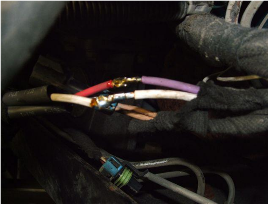
Figure 5. Harness Splice Crimped and Soldered
