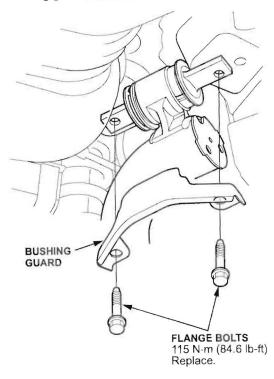
6. Remove the flange bolt from the rear mount of the trailing arm. The bolt will not be reused.
