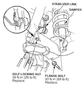
4. Remove the flange bolt from the lower mount of the damper, then detach the damper from the trailing arm. The bolt will not be reused.
