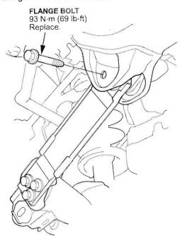
7. Lower the floor jack, and remove the trailing arm.
