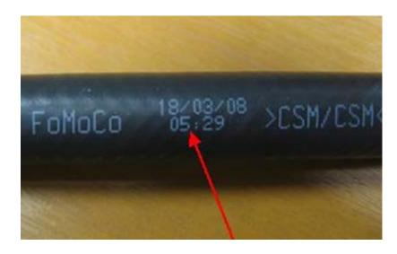
The manufacturing date and time on **both** sections of rubber hose on the return line must be checked.
