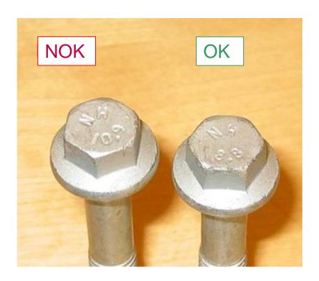
Check the marking on the screw heads.
