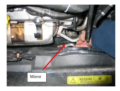
Check the markings on the screws using a mirror and flashlight. If the screws are of the correct specification, reinstall components in reverse
