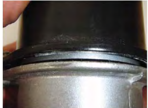
INSIDE OF CASE IS CLEAN (Install cover kit only. Do not install motor kit.)
