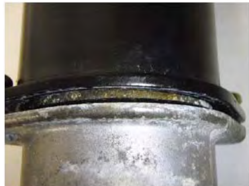
INSIDE OF CASE IS CORRODED (Install motor kit only. Do not install cover kit.)
