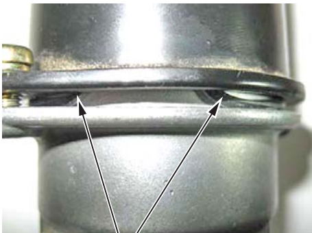
NO GOOD O-ring is pinched and/or rolled.
