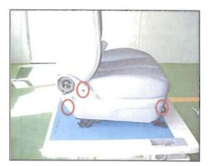
NOTE: When removing the side outer cover, verify the clip (p/n 88173-3K000) is installed on the outer cover. If the clip remains lodged on the seat bracket, remove it and install it onto the side outer cover.
