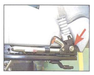
Raise the front seat and disengage the 2 seat covering fixing hooks on the bottom side of the seat.
