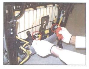
8. Disconnect the OCS wiring connector and disengage the 2 wiring clips.
