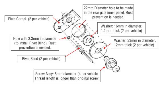
(k) Take 2 Washers (16mm and 33mm in diameter) from the kit and combine them with a new Stud Bolt. The 2 washers should be installed in proper order, as indicated in the illustration above. Tighten the stud bolt to the plate. (Torque spec 4.5+0.5 ft.lb.  $(19.6 \pm 6 \text{ Nm or } 2.0 \pm 0.6 \text{ kgf-m}))$
