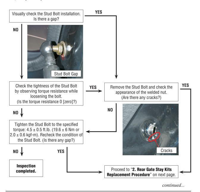
Note: Never disassemble the rear gate stay or separate the stud bolt from the stay.
