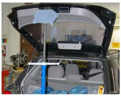
(b) Using a 12mm open end wrench, remove the rear gate stay by unfastening both the upper and lower stay stud bolts. Note: On some models it will be necessary to remove the lower trim panel found around the lower stud bolt.
