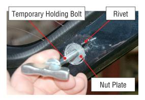
(i) Align the rivet hole in the Nut Plate with the 3.3mm hole in the tailgate. Insert the blind rivet through the tailgate and into the plate. Align and center the hole in the Nut Plate within the 22mm hole. Be sure the Nut Plate is flush against the inner wall of the tailgate. Using a rivet gun, permanently fasten the rivet.
