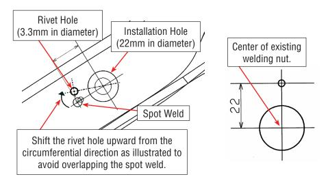
Caution: The wire harness for the rear window defroster is located within the area of the tailgate to be drilled. To avoid damaging the harness, be careful not to drill deeper than necessary.
