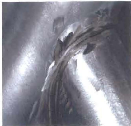
After the stainless steel wire brush procedure, slowly cut into the tubing and the weld (not the neck)
