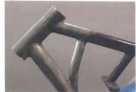
View showing the two new welds
