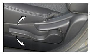
Raise the driver's seat (shown) to its highest point using the seat height adjustment lever. Pump the lever several times until the seat stops at its highest position.
