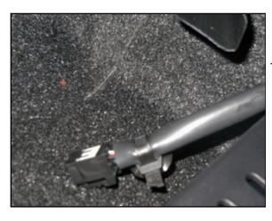
7. Attach the tie strap (MU800001) to the harness approximately 1/4" (5mm) from the end of the harness shielding as shown. Cut the excess from the tie strap and discard it.
