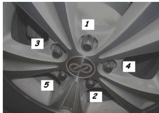
Figure 2. Torque wheel nuts in the order shown.
