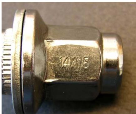
Figure 1 Identifying wheel nuts requiring replacement
