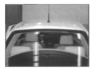
Remove spoiler from packaging and dry fit spoiler onto vehicle to ensure alignment of spoiler is not more than 1 mm from edge on each of the three sides
