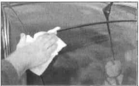
← Clean area of window where spoiler will make contact with glass using isopropyl alcohol wipes - allow five minutes to dry
