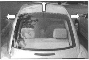
← Ensure alignment of spoiler is not more than 1 mm from edge on each of the three sides
