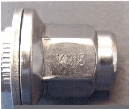
Figure 1 Identifying wheel nuts requiring replacement
