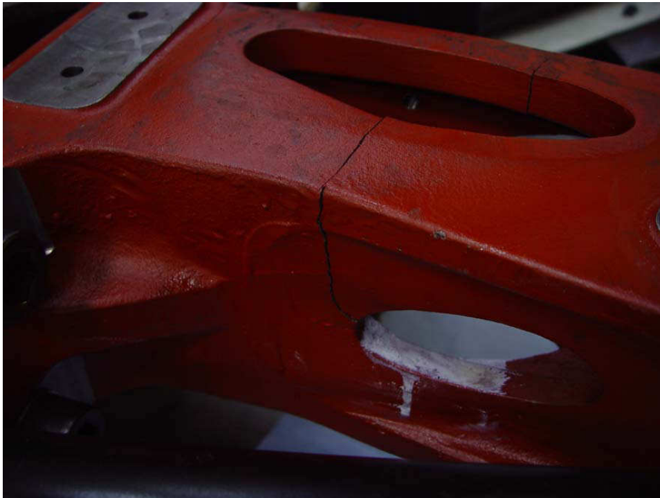
Cracks in the rear casting after 210,000 reversals
