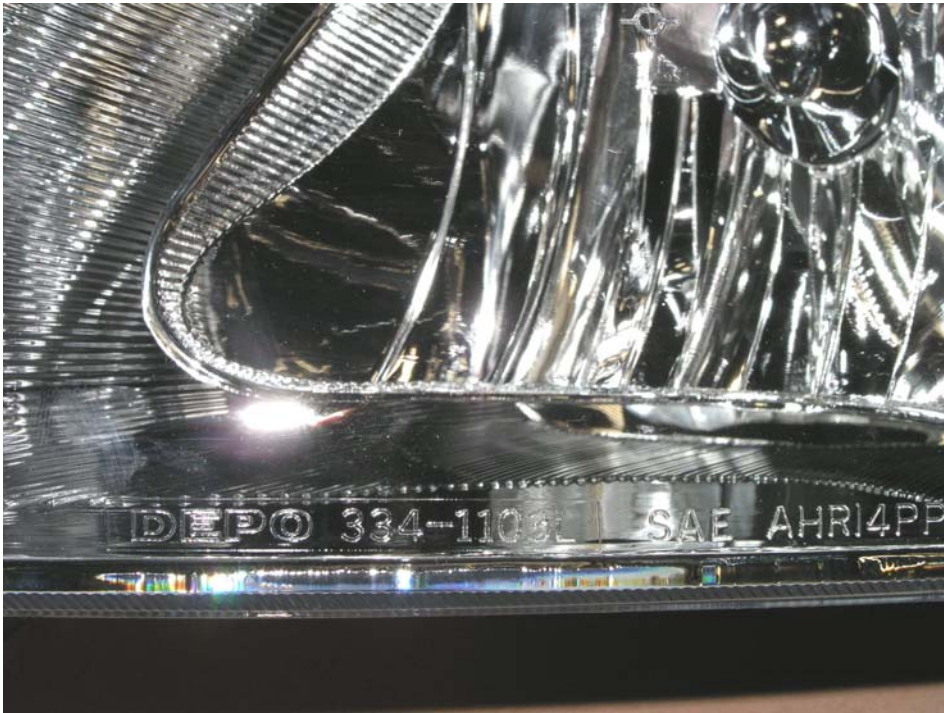
DEPO logo and part number on lens. Note: 334-1103L (left hand side lamp) shown above. The part number for right hand side lamp on the lens is 334-1103R.
