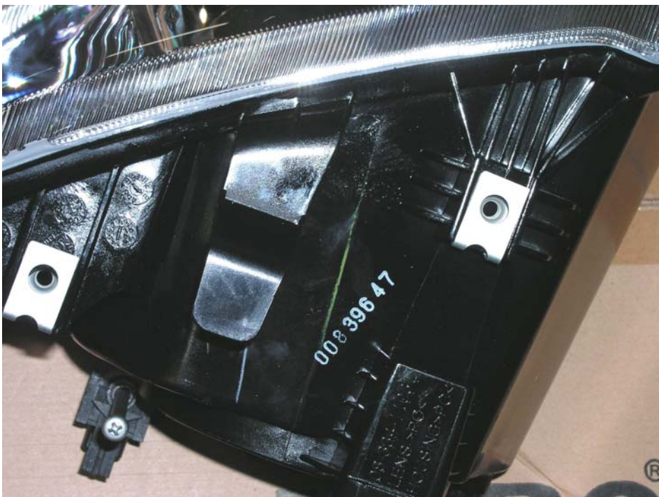
DEPO production lot number on the top side of housing.
