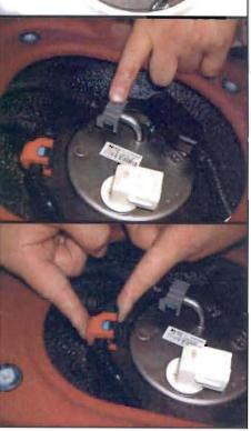
NOTE: The rear connector body must be attached to the holding bracket tab of the fuel pump top plate.
