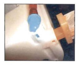
24. Reconnect the fuel sender wiring connector.
