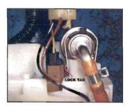
Carefully insert the reworked fuel pump complete assembly into the fuel tank access opening.
