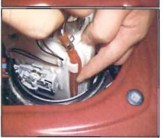
Reinstall the fuel pump plate cover (H) and tighten it down fully using the SSTJ-48889 (G).
