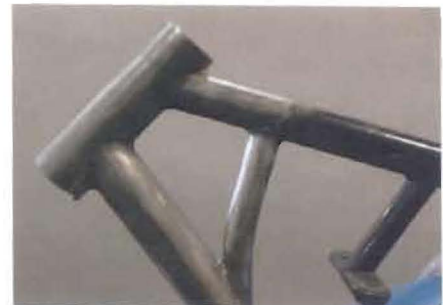
View showing the two new welds
