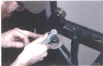
Remove frame paint/powder coating from around the repair area
