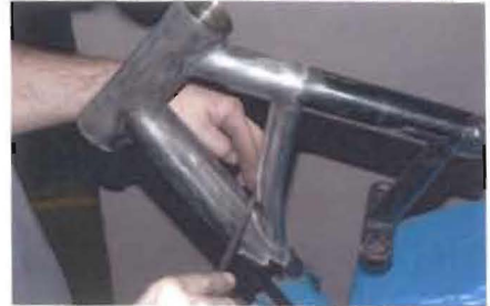
Use a file or hacksaw blade to remove any residual coating and finish with a stainless steel wire brush
