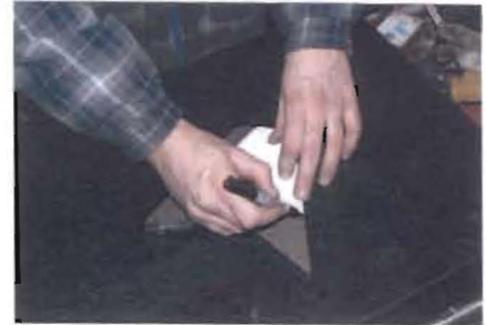
Transfer the profile of the template to the 1/4" thick plate using a permanent marker as shown
