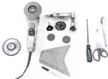
Recommended hand tools and gusset that will need to be trimmed
