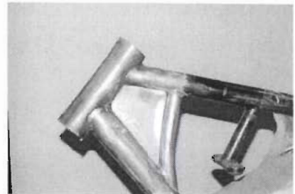
Position the plate in in the opening along the centerline of the tubes.
