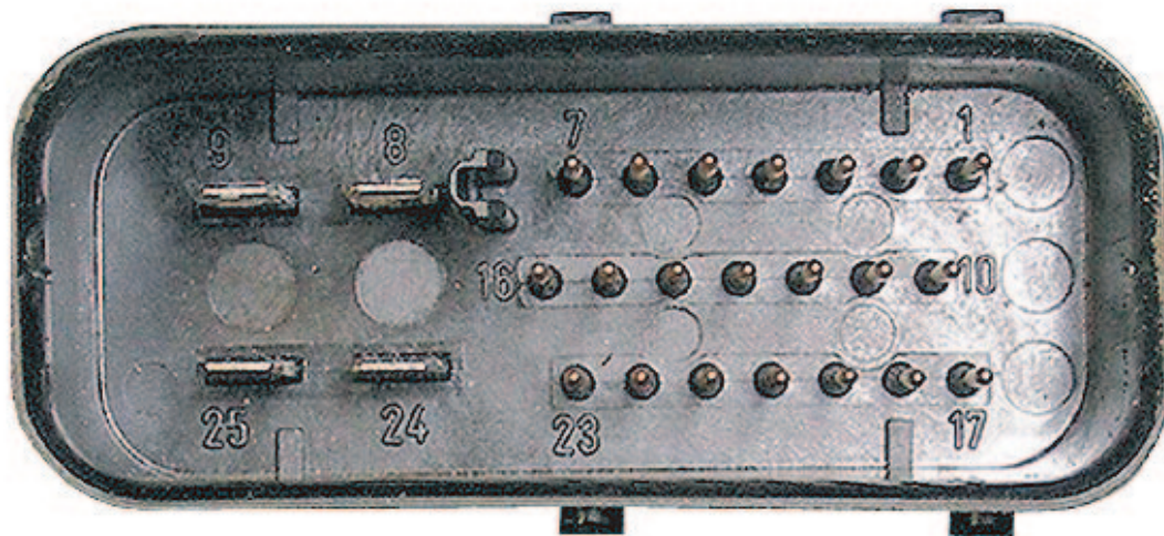
INSPECT CONNECTOR FOR ANY SIGN OF CORROSION
