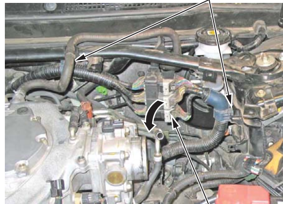
ENGINE HARNESS (Rotate out of the way.)
