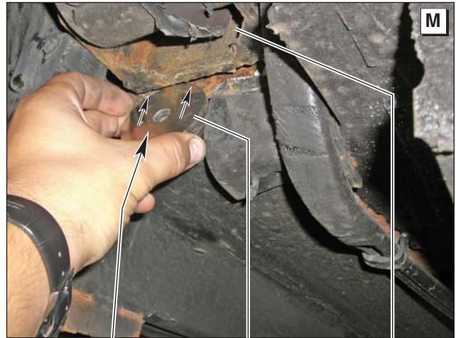
Insert body washers in gap. Body Washers (Spacers) Rear Axle Mounting Bracket
