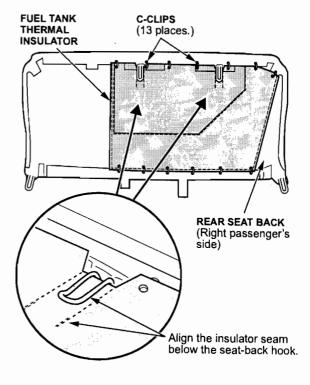
4. Using upholstery (hog) ring pliers and C-clips, attach the insulator to the seat-back at each of the pre-punched holes. Make sure you attach each clip to the metal part of the seat frame. Don't remove the existing seat cover clips.
